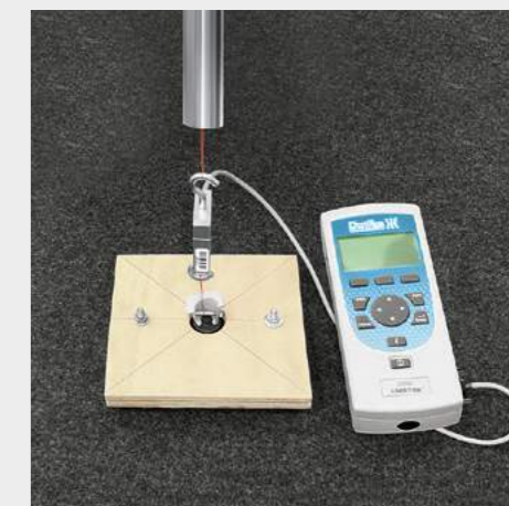
Testing of fixing element strength
